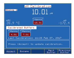
Up to five-point pH calibration with automatic buffer recognition
