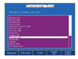
Selectable ISEs preprogrammed with molecular weight and ion charge
